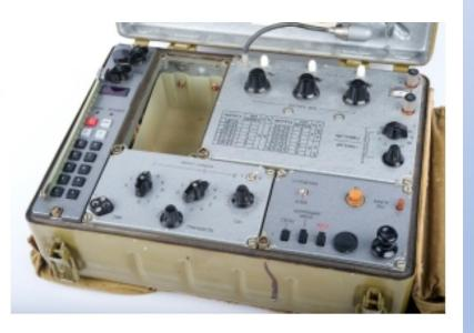
At least two different versions of the R-394K are known, both of which are extremely rare. The oldest one has an analogue burst encoder that uses magnetic tape, whilst a later one has a digital burst encoder. The latter is shown above and was short-lived. It can be seen as an intermediate step towards the design of the fully digital military R-394KM and the R-394T agent version.
